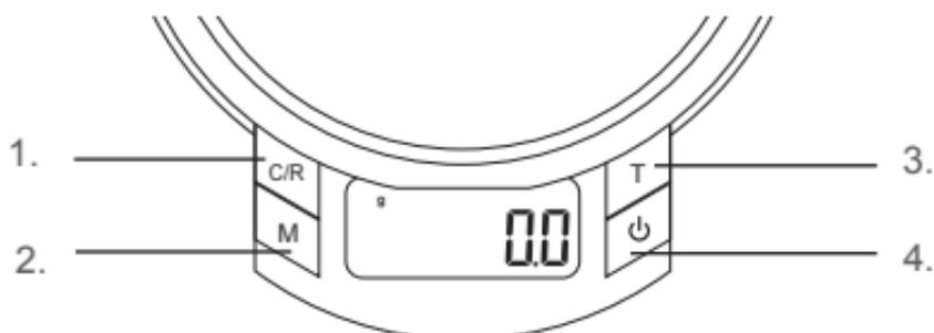
1. **C/R Key** - Tap to enter Counting Mode. Hold to set the piece weight and sample size.
